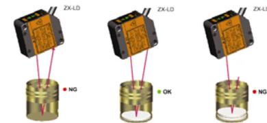
Determine the number of inner linings deposited in bottle caps with a laser measurement sensor. The judgment output of the amplifier can be used to eject unacceptable caps before they get reach the capping machine.
