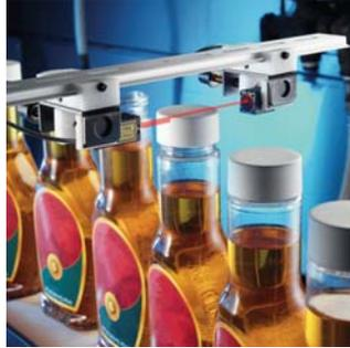
Use a single measurement sensor to detect multiple bottle cap application problems. Get 100% in-line inspection at full production speeds and accurately detect these defective capping conditions:
