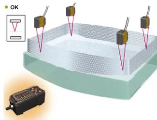
Confirm proper installation of a shadow mask into CRTs using line beam laser measurement sensors at each corner to ensure proper insertion depth.
