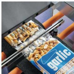
Detect improper seals from product obstruction in Form, Fill & Seal machines. Product mis-feeds in vertical or horizontal form, fill and seal machines often result in the product being pinched between the sealing jaws at the seams of the package or pouch. If not detected quickly, this type of "jam" can result in significant loss of product and packaging because the condition that caused it continues to create jams until it is corrected.
