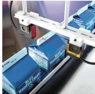
Inspect seals on gable-top cartons regardless of product position using two laser measurement sensors and a calculating unit. Prevent spillage and spoilage from improperly sealed cartons that lead to wasted product and added machine cleaning costs. If spoiled product reaches the supply chain, it can lead to loss of consumer confidence and product recalls.
