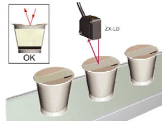
Detect vacuum under lids of jars and dairy cups by measuring the concave shape on acceptable products and flat surface on unacceptable ones. The raised or flat safety button on jar lids indicates an imperfect seal and lost vacuum. A flat foil lid on a dairy cup indicates vacuum lost through a pinhole or other seal imperfection.
