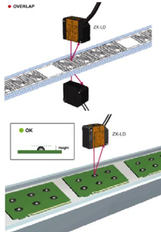
Detect overlapped lead frames and other shiny metals. The laser measurement sensor detects metal plates just 0.15 mm thick.
