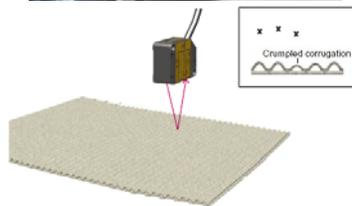
Detect crumpling or weakened corrugations in cardboard packaging materials as sheets move along a conveyor. The laser measurement sensor inspects each corrugation for uniform height.
