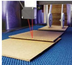
Detect double feeds of cardboard sheets into case formers. Use a laser measurement sensor to prevent jamming and reduce wasted packaging material. The problem is usually associated with variations in the cardboard density or environmental conditions such as excessive humidity that makes the stacked blanks stick together.
