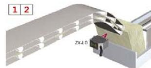
Count sheets of wrapping paper with laser measurement sensor detecting stack thickness.
