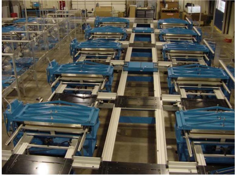
The PowerPallet-equipped production line at Hexcel Manufacturing features semi-autonomous carts exchanging data via wireless DeviceNet.
